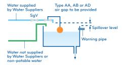
Please note if water is drawn via this arrangement for wholesome water purposes then all pipework and points of use downstream of this arrangement must also comply with the Water Regulations.
