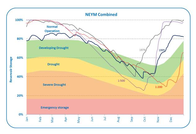
Figure 2 - NEYM Combined Reservoir Drought Action Zones showing the results of scenario testing
