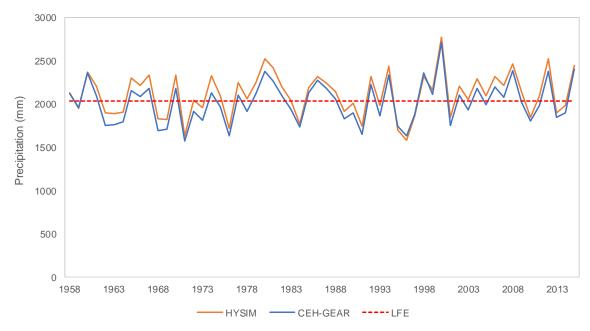
Figure 4.22 - Annual precipitation for the Afon Dwyfor at Dolbenmaen catchment calculated based on: precipitation extracted from HYSIM, CEH-GEAR dataset and LFE
