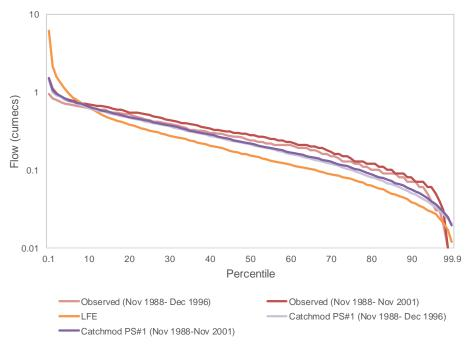
Figure 4.17 - Flow duration curves for Cwmystradllyn reservoir catchment based on observed and simulated streamflow
