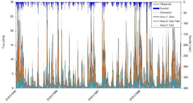
Figure 6.17 - Contribution to flow by area for Marchlyn Bach catchment using Catchmod simulated flows (drought detail)
