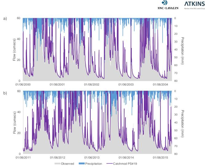
Figure 5.6 - Observed and simulated streamflow for Afon Teifi at Glanteifi with foccus on low flows for two time periods: a) June - December 2004; b) June 2012 - December 2013
