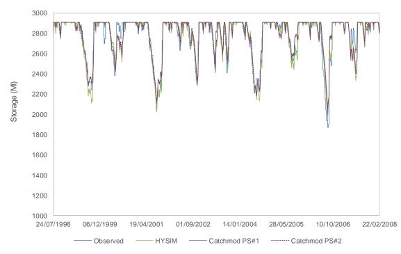
Figure 4.20 - Llyn Cwmystradllyn observed and modelled storages. As per AFW (2017), the modelled storages in this figure were calculated using fixed compensation and regulation amounts (abstraction rate =13 Ml/d and compensation release =4 Ml/d).
