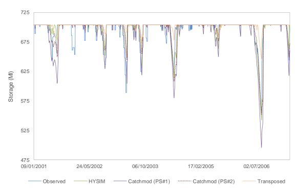
Figure 4.12 - Llyn Cwm Dulyn observed and modelled storages, including flow transposed from Llyfni at Pont Y Cim catchment
