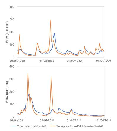
Figure 5.4 - Two distinct time periods showing how different transposed flows from Ddol Farm to Glanteifi (transposition factor based on ADF) are from observed flows at Glanteifi
