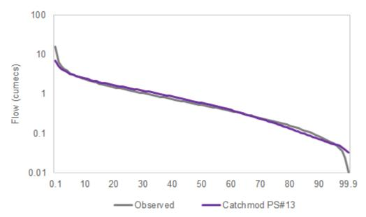
Figure B.7 - Llanrhystud FDC for observed flow and FDC for the Catchmod calibration (for parameter set #13)
