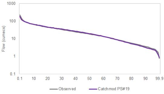
Figure 5.7 - Flow Duration Curves for observed flow and for the Catchmod calibration (for parameter set #19)
