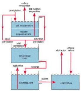
Figure 2.1 - Catchmod schematic. Image from Wilby et al., 2006.
