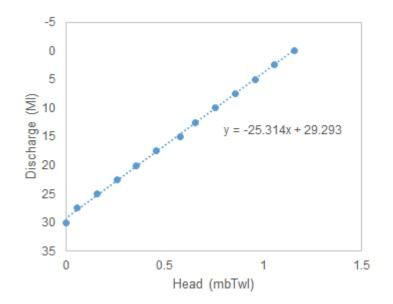
Figure 5.14 - Head/Discharge relationship for Pond y Gwaith (plot provided by DCWW)
