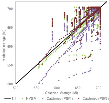
Figure 4.10 - Llyn Cwm Dulyn observed against modelled reservoir drawdown for HYSIM and Catchmod calibration. Data shown here covers the time period between 13/01/2001 and 20/04/2007 to be consistent with the time period selected by AFW (2017).
