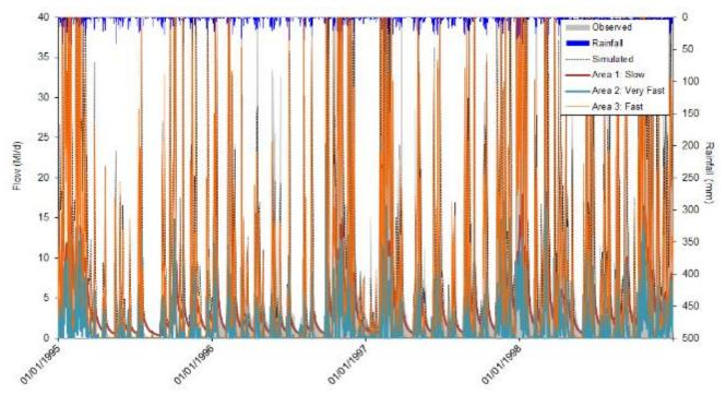
Figure 6.16 - Contribution to flow by area for Llugwy catchment using Catchmod simulated flows (drought detail)
