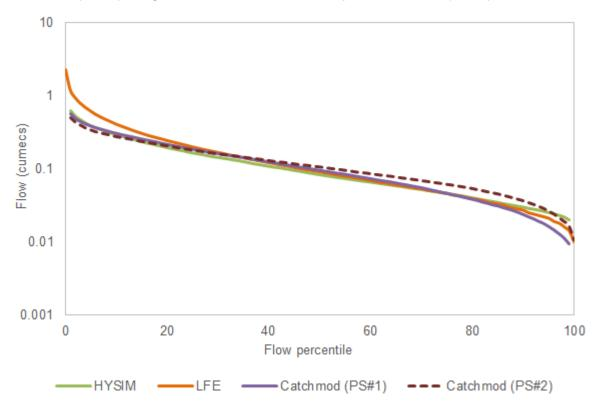
Figure 4.6 - Flow Duration Curves for the HYSIM calibration, for the Catchmod calibration (for two distinct parameter sets, #1 and #2) and from LFE
