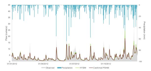
Figure 4.24 - Simulated and observed naturalised flows for Afon Dwyfor at Dolbenmaen
