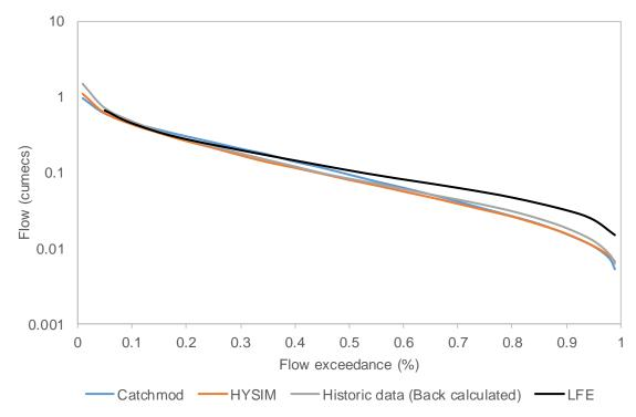
Figure 6.5 - Flow Duration Curves at Ffynnon Llugwy for Catchmod, HYSIM, historic data (back-calculated) and from LFE.
