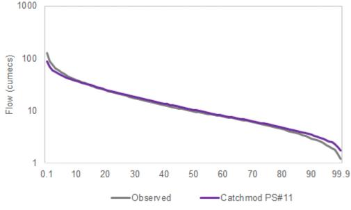
Figure B.4 - Llanfair FDC for observed flow and FDC for the Catchmod calibration (for parameter set #11)
