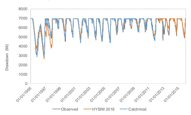
Figure 6.18 - Water balance fit for Alaw reservoir (Observed, Catchmod simulation and HYSIM 2016 simulation)
