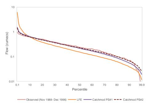
Figure 4.18 - Flow duration curves for Cwmystradllyn reservoir catchment based on observed and simulated streamflow
