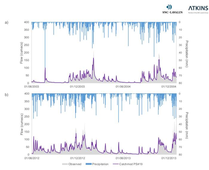
Figure 5.5 - Observed and simulated streamflow for Afon Teifi at Glanteifi for two time periods: a) June - December 2004; b) June - December 2013
