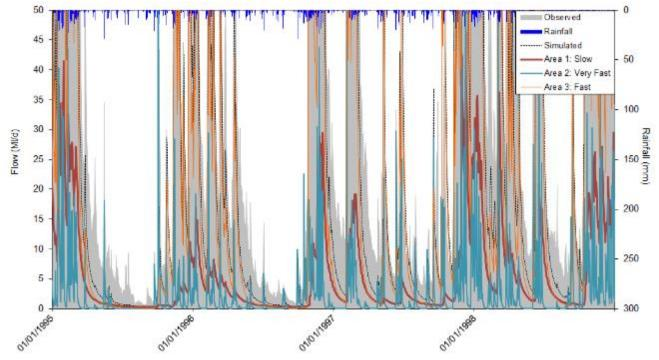
Figure 6.13 - Contribution to flow by area for Alaw catchment using Catchmod simulated flows (1990s detail).
