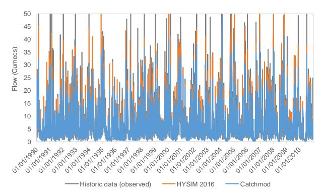
Figure 6.12 – Observed and simulated (HYSIM 2016 and Catchmod) flows for Glaslyn.
