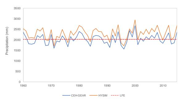
Figure 4.14 - Annual precipitation for the Cwmystradllyn catchment calculated based on: precipitation extracted from HYSIM, CEH-GEAR dataset and LFE
