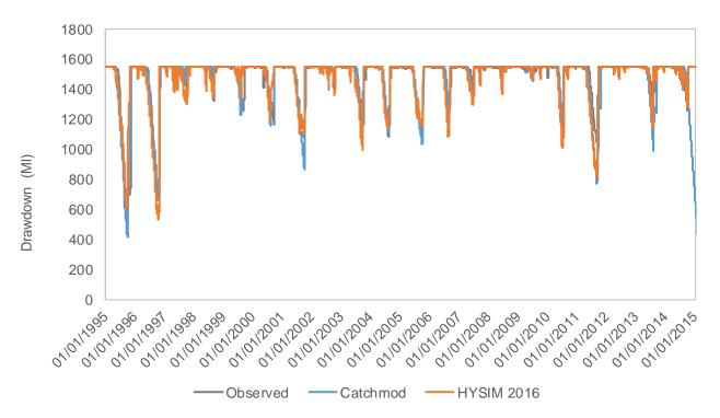
Figure 6.19 - Water balance fit for Cefni reservoir (observed, Catchmod simulation and HYSIM 2016 simulation)
