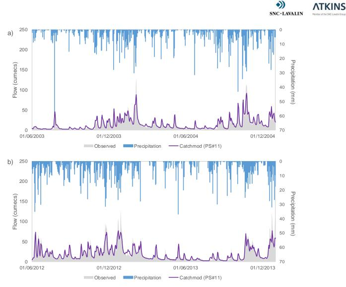
Figure B.3 - Llanfair observed and simulated streamflow for a) 06/2003-12/2004; b) 06/2012-12/2013
