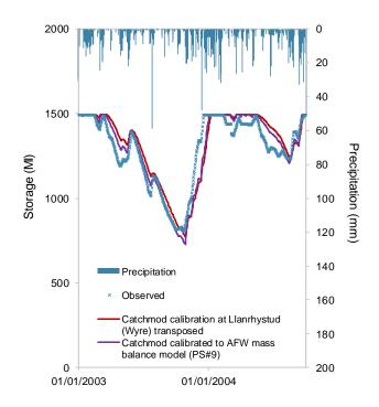
Figure B.12 - Observed and modelled storages for Teifi Pools for 01/2003-09/2004, using a constant transfer from Pond y Gwaith of 2.00 MI/d throughout 2003, and 3.11 MI/d during the rest of the time.
