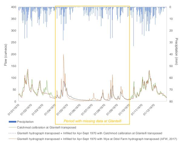
Figure 5.9 - Simulated flow at Llechryd by transposition of observed flow at Glanteifi and by transposing Catchmod calibrated at Glanteifi
