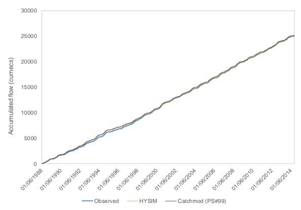
In terms of volumetric fit both models perform equally well (Figure 4.25).
