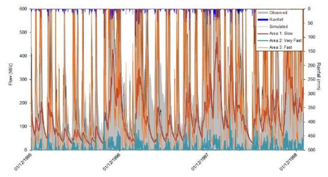
Figure 6.15 - Contribution to flow by Area for Glaslyn catchment using Catchmod simulated flows (drought detail)
