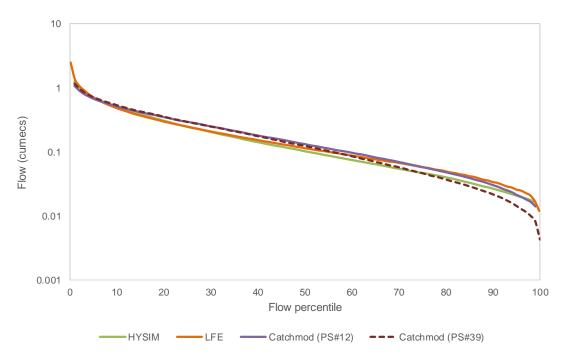
Figure 3.6 - Flow Duration Curves for the HYSIM calibration, for the Catchmod calibration (for two distinct parameter sets, #12 and #39) and from the LFE
