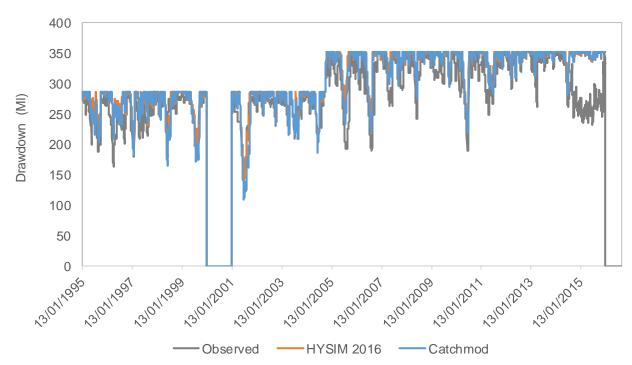
Figure 6.21 - Water balance fit for Marchlyn Bach (observed, Catchmod simulation and HYSIM 2016 simulation)
