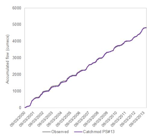
Figure B.8 - Volumetric fit for Wyre at Llanrhystud
