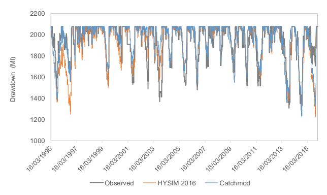
Figure 6.20 - Water balance fit for Ffynnon Llugwy (observed, Catchmod simulation and HYSIM 2016 simulation)
