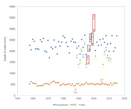
Figure 4.15 - Annual values calculated based on data extracted from HYSIM files. The numbers in the plot represent the number of days with missing flow data in each year when calculating the flow annual value. For days with missing data, the flow was assumed to be equal to zero, when calculating the annual value.
