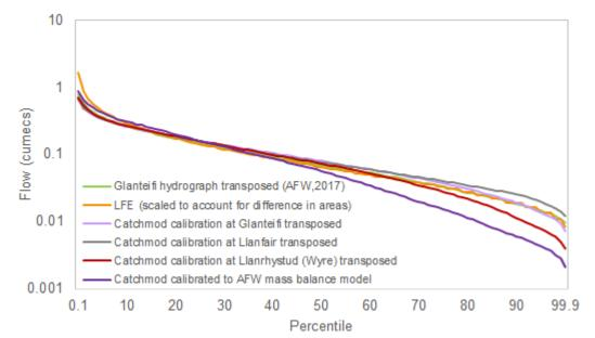
Figure B.9 - Flow Duration Curves from the LFE, for the Catchmod calibration transposed from Llanfair, Glanteifi and Llanrhystud (Wyre), for the Catchmod calibration using the mass balance model (parameter set #9) and for Glanteifi hydrograph transposed.
